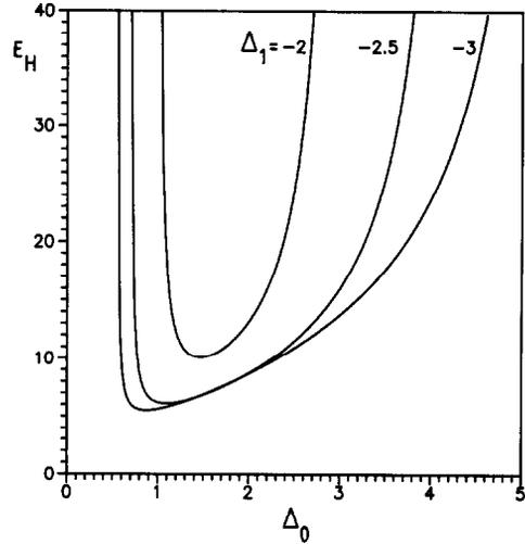
Fig. 1. Limits of stability of the steady state solutions. The boundaries correspond to the locus of Hopf bifurcations as given by eqs. (5) for  $\gamma = 1$ .
