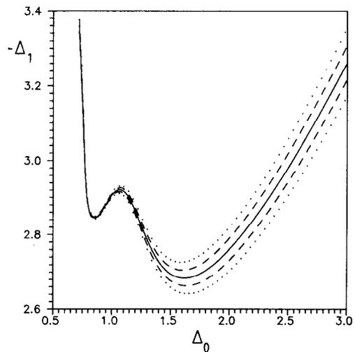
Fig. 2. Contour lines in the  $(A_0, A_1)$  plane for  $\gamma=1$ . From top to bottom, the five lines are the solutions of  $E_2 = F(\gamma, A_0, A_1) = 0.4, 0.2, 0.0, -0.2$  and  $-0.4$ , respectively. For each set of parameters, the domain above the contour line is a domain of supercritical Hopf bifurcation.
