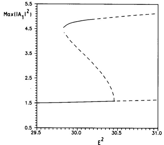
Fig. 5. Example of bifurcation diagram with a subcritical Hopf bifurcation at  $E_H=5.519$  for  $\gamma=1$ ,  $\Delta_0=0.83$  and  $\Delta_1=-3$ . The hysteresis exists in the domain  $5.46 < E < 5.519$ . The stable periodic solution on the upper branch becomes unstable at  $E=5.493$ .
