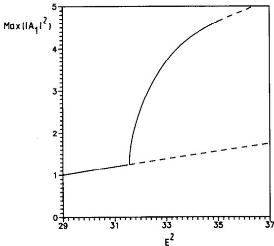
Fig. 4. Example of bifurcation diagram with a supercritical Hopf bifurcation at  $E_H=5.62$  for  $\gamma=1$ ,  $\Delta_0=1$  and  $\Delta_1=-3$ . The graph represents the maximum of the subharmonic oscillation amplitude versus the input field intensity. Full lines correspond to stable solutions. The periodic solution becomes unstable at  $E=5.907$  via a period doubling bifurcation.
