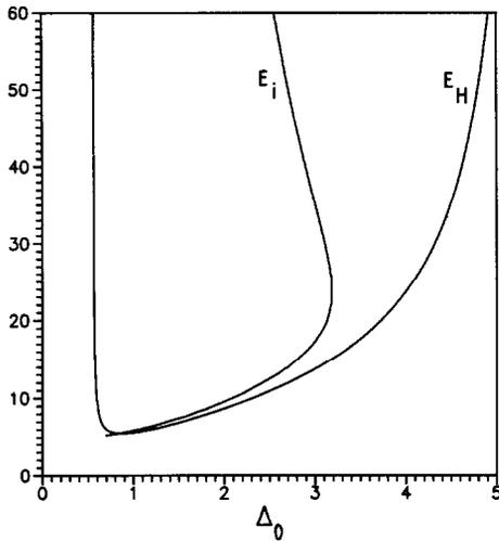
Fig. 3. Boundaries for the stability of the steady state solution ( $E_H$ ) and the periodic solution ( $E_i$ ) for  $\gamma=1$  and  $\Delta_1=-3$ .
